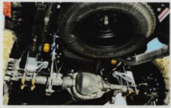
A Blocks lift the rear end of the Super Duty kit, though McGaughy's does have a full spring option if you want to go that route. You do not have to worry about these blocks spitting out, though, as they are retained by the inner U-bolts thanks to the design of the welded-plate blocks.
