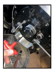
IF NEEDED REMOVE & CLEAN BEARING IN SOLVENT & REINSTALL\* (\*TO REMOVE SEE PDF ON REPLACING FRONT BEARING)
