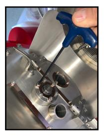
ONCE COVER IS REMOVED YOU MAY WANT TO CLEAN OLD GREASE NEXT PACK BEARING WITH FRESH GREASE & REPLACE WITH COVER
