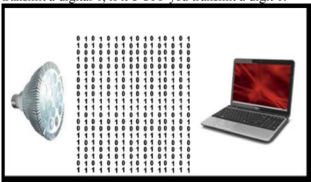
Fig.2: Basic Principle of Li-Fi Technology
