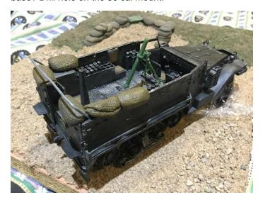
Here's my first attempt at airbrushing with acrylics, plus dust. Note, wind screen was clear plastic packaging. Added netting on helmet and used Tamiya masking tape for straps on helmets. Added the missing aerial base and stretched spur for aerial.
