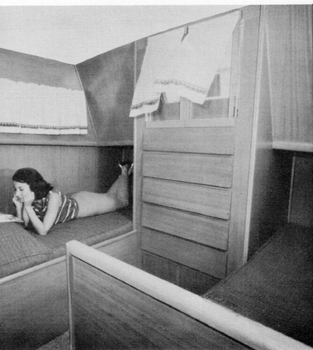
Master stateroom has built-in drawers beneath screened windows to an escape hatch. Built-in bunks have polyfoam mattresses. Four 110-volt outlets. Large hanging clothes locker.
