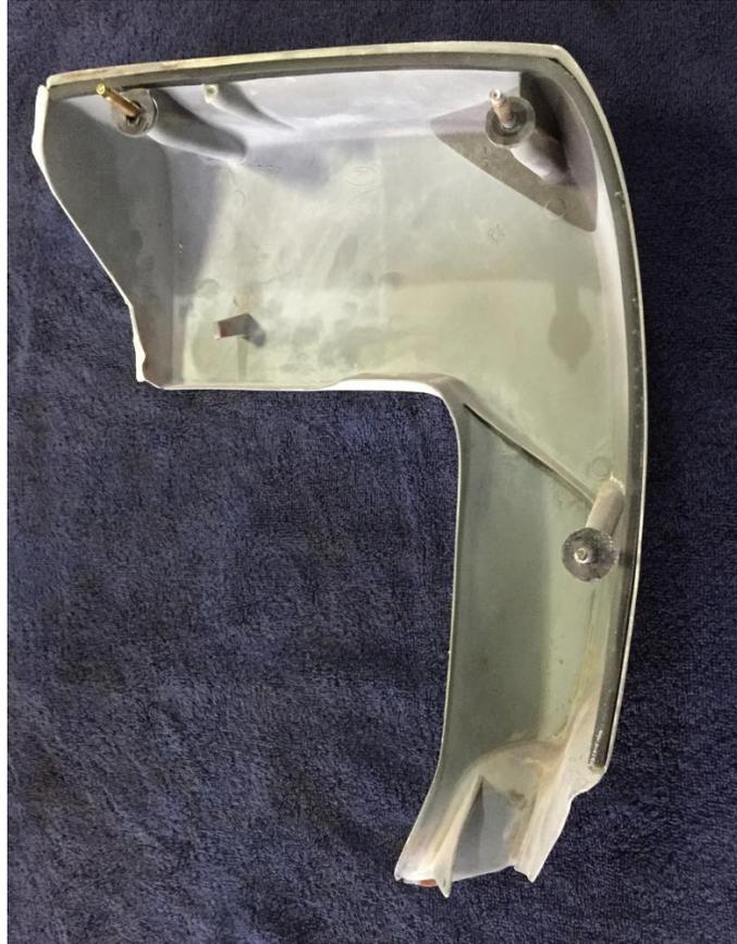
In the picture at left, the rubber strip seal is installed on the quarter panel extension. Notice each stud also has a rubber washer seal. Thus, when installed, there's a rubber washer on both sides of the taillight panel to ensure a good seal for keeping water out of the trunk. More importantly, these seals also keep exhaust fumes from entering the trunk and, eventually, the passenger compartment.
