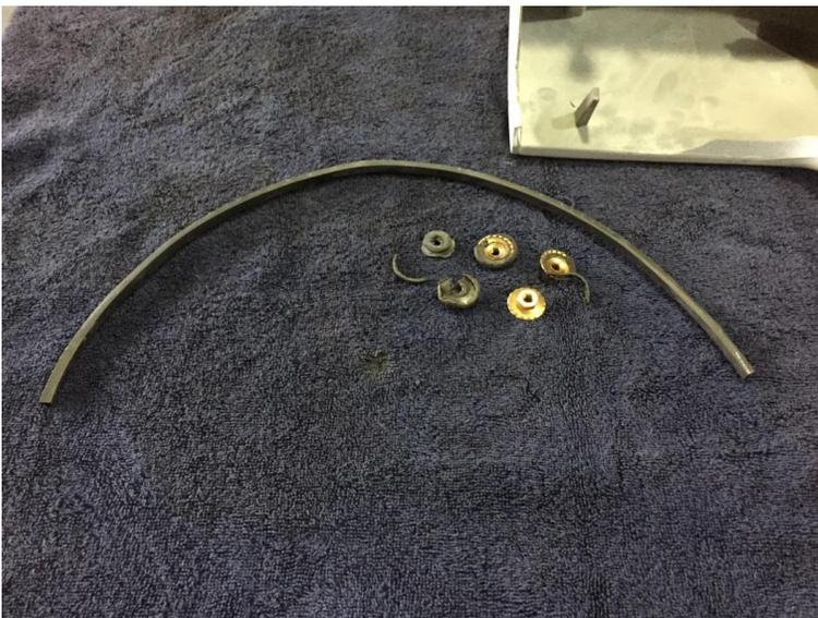
Here you can see the rubber strip seal from one of my quarter panel extensions. Not only does it help to keep moisture from collecting, it actually makes adjusting these parts much easier. I also ordered new fasteners from AMK. The nuts have rubber washers attached, but they are extremely soft and very delicate. I learned the hard way they can be installed only once. Removing them destroys the attached washers. I'll have to order another set for final assembly.
