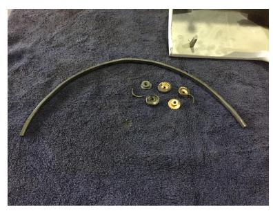
Here you can see the rubber strip seal from one of my quarter panel extensions. Not only does it help to keep moisture from collecting, it actually makes adjusting these parts much easier. I also ordered new fasteners from AMK. The nuts have rubber washers attached, but they are extremely soft and very delicate. I learned the hard way they can be installed only once. Removing them destroys the attached washers. I'll have to order another set for final assembly.
