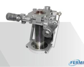
This compact XYZ Stage provides precise motion and manipulation of samples inside ultrahigh vacuum environments. Mounting flanges are available in NW38CF or NW63CF flanges. Edge welded stainless steel bellows is used to allow the NW38CF flanges to travel within limited range.
