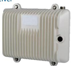
The CRX2 is powered via a single cable and sends the MPEG Transport Stream over IP, either by Ethernet cable or over ruggedized fiber, to a computer-based software or hardware decoder. The CRX2 system automatically optimizes the receive signal, and virtually eliminates all human intervention.
