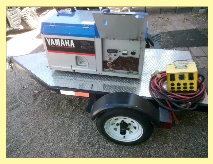
his 6,500 watt single phase generator is diesel powered and mounted on a small 2 wheel trailer with a 2" hitch for easy towing. It has the convenience of a very low profile so it is easy to hide from view. It is an extremely quiet running unit powered by a Kubota diesel engine.
