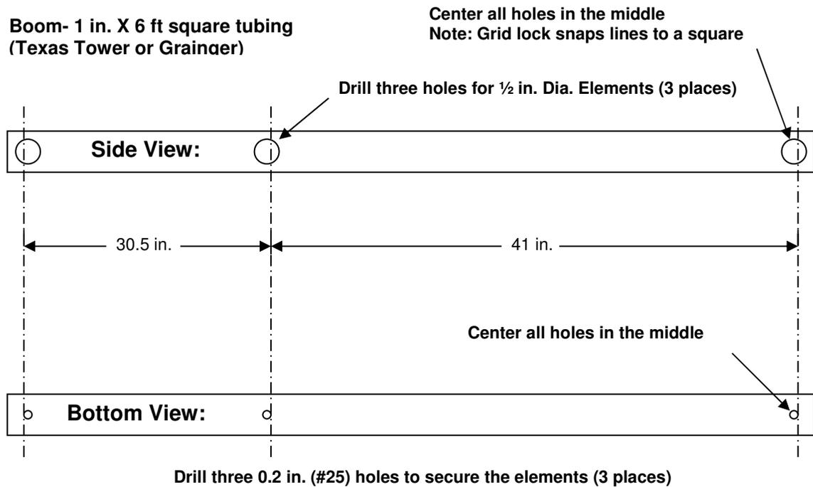
**Figure 2.** Dimensions for the mounting holes required for 1 in. X 6 ft square boom preparation.
