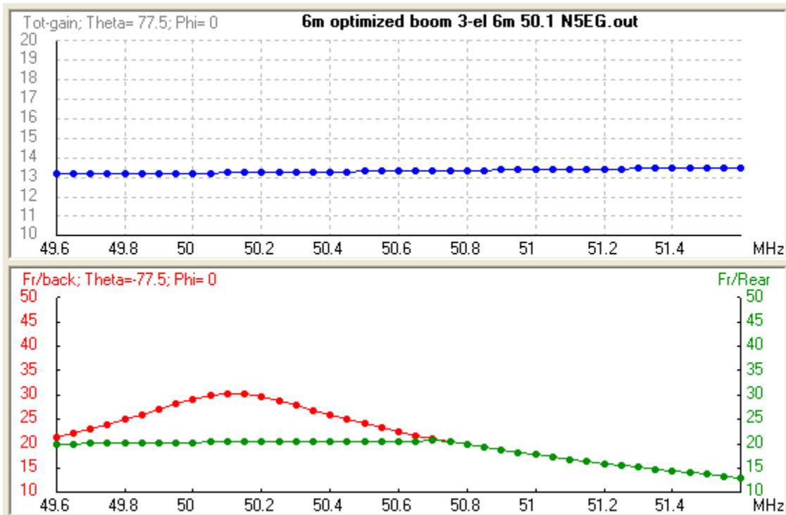
**Figure 1.** Gain and front-to-back curves show the design over a wide bandwidth.
