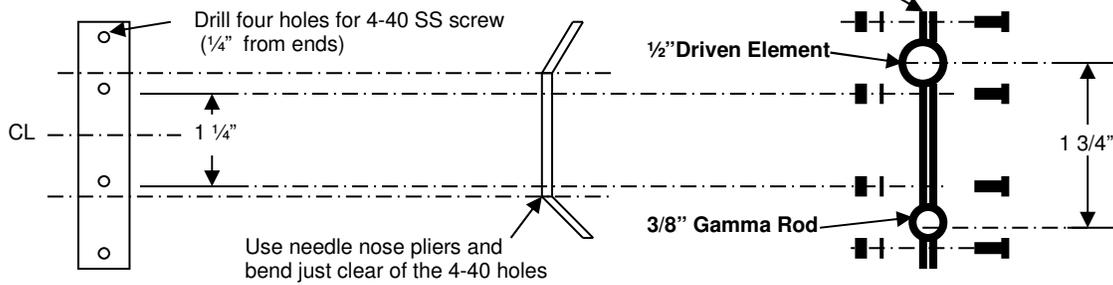
**Figure 4.** This illustration shows details to fabricate the Gamma match assembly.
