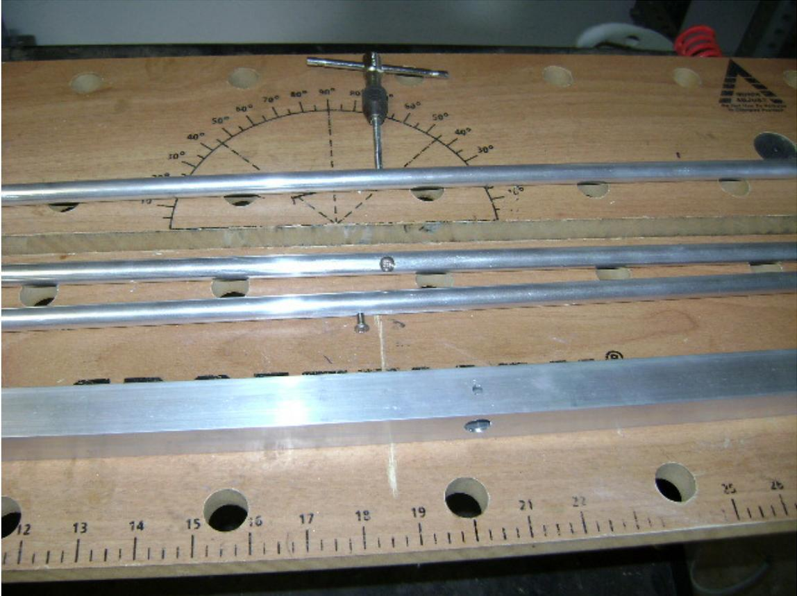
**Figure 5.** Yagi Assemblies showing a boom hole and element holes that have been tapped for 8-32 screws.
