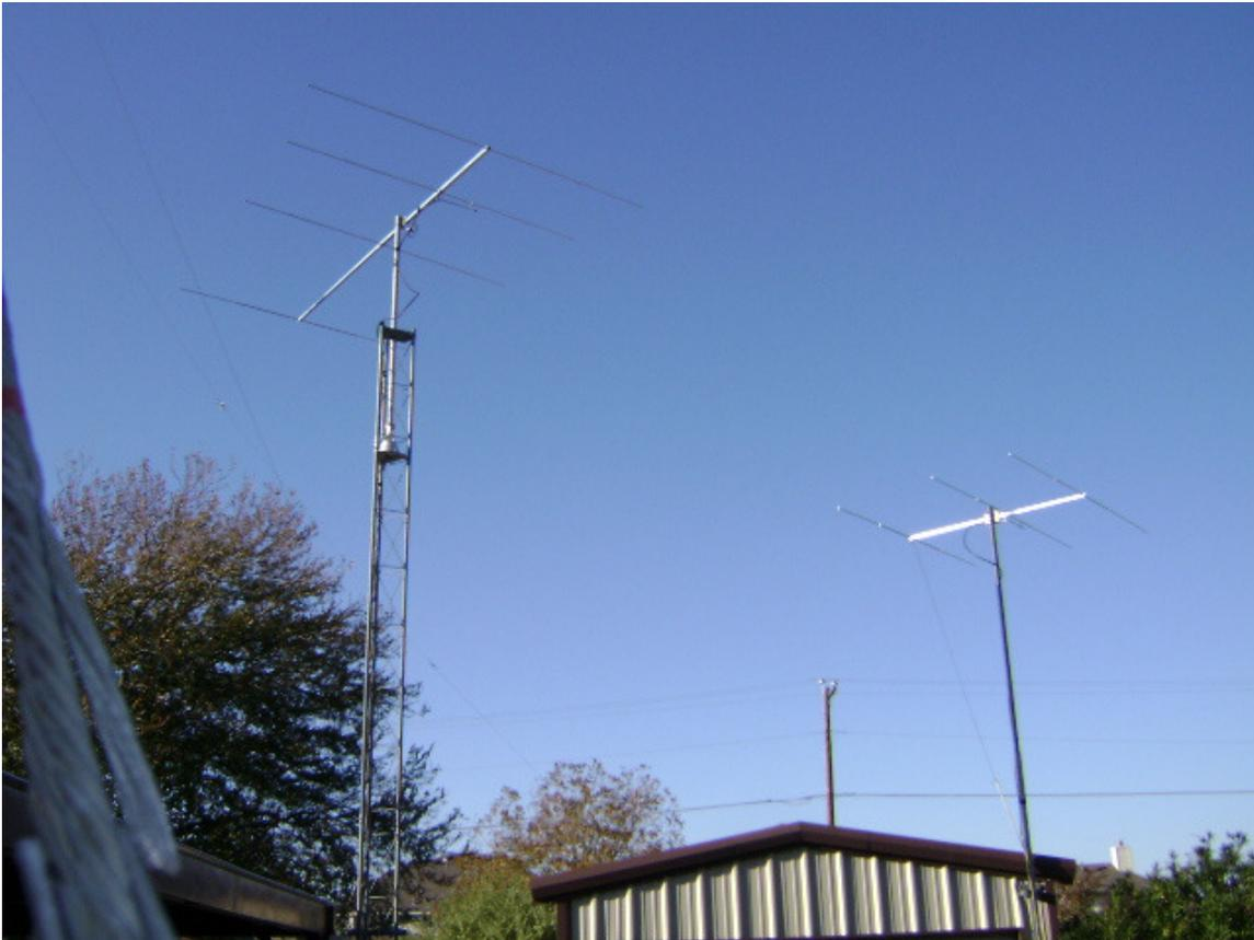
**Figure 9.** This plumber's delight six-meter yagi being compared and tested against my four element yagi with great signal gain and front-to-back patterns.
