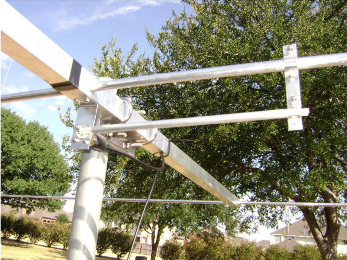
**Figure 8.** Adjust the yagi for minimum SWR above ground as high as possible.
