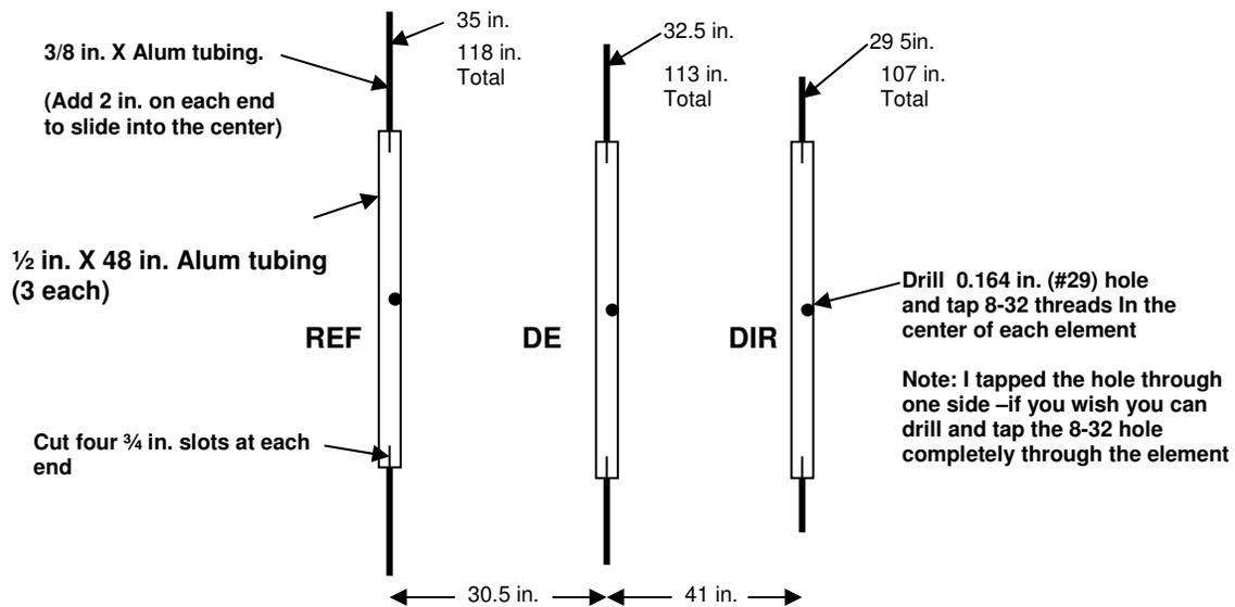
**Figure 3.** This illustration shows element construction.
