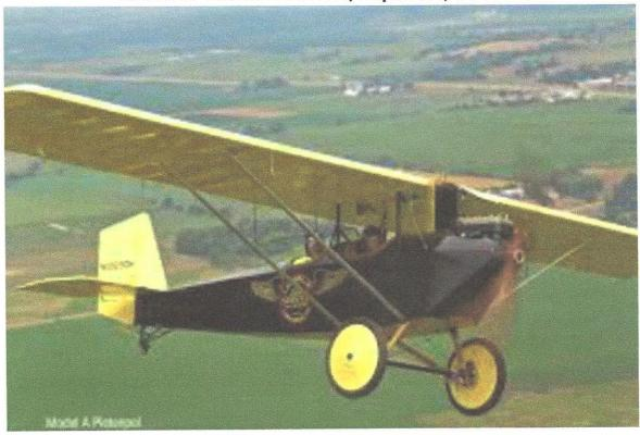
The Pietenpol Air Camper is a simple parasol wing homebuilt aircraft designed by Bernard H. Pietenpol. The first prototype that became the Air Camper was built and flown by Pietenpol in 1928. Wingspan: 29'0" Top speed: 99 mph Length: 17.68 Engine type: Ford Model A. Gar Williams of the Naper A's has one of these aircraft and will show it to us this Saturday.
