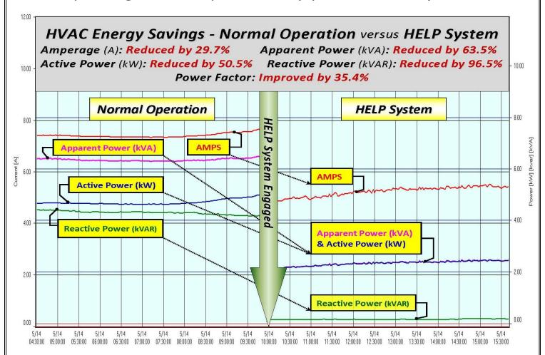
At 10:00 AM, (Green Arrow) we switched-on the HELP System to resume operational testing. The Right-hand section of this chart shows the next six hours of operation with the HELP System in operation.
