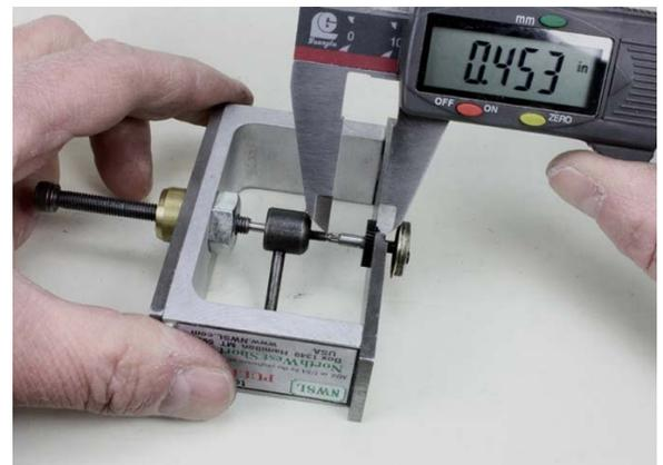
13. The worm should already be pressed onto the shaft of the motor provided in the kit. Use the Quick Mount provided to position and hold the motor on the frame so that the worm and worm gear mesh tightly. Make sure the motor shaft and worm are parallel with the worm gear and that the mesh of the worm and worm gear is centered on both gears. Centered and square!
