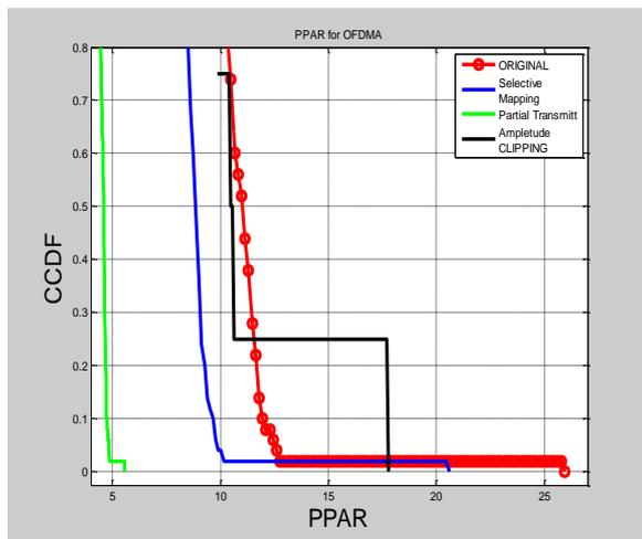
Fig.10: PAPR of OFDMA from different scheme
