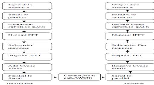
Fig.5: Transmitter Receiver systems for SC-FDMA
