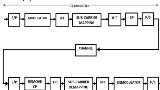
Fig.4: Block diagram of the SC-FDMA system model
