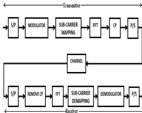
Fig.2: Block diagram of the OFDMA system model
