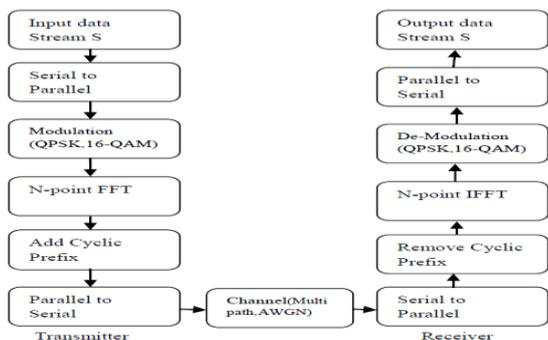
Fig.3: Transmitter Receiver system for OFDM
