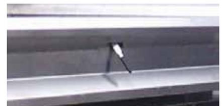
Fold down sides feature a centrally located quick release lever that extends and retracts ¾" pins at each end using a solid linkage member. Weight-saving aluminum fold down sides are optional on steel bodies.
