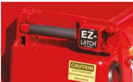
Rugby's patented and industry leading EZ-LATCH™ (located on each side of body) allows for easy body access. The latch system is designed for quick opening and slam lock operation with a cam action to draw-in upper tailgate pins.
