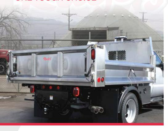
Stainless steel dump bodies from Rugby are corrosion resistant and more durable than high tensile steel. The polished bodies offer a modern, bright, easily maintained and attractive appearance.
