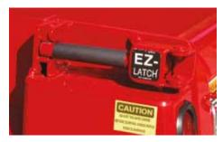
Rugby's patented and industry leading EZ-LATCH™ (located on each side of body) allows for easy body access. The latch system is designed for quick opening and slam lock operation with a cam action to draw-in upper tailgate pins.
