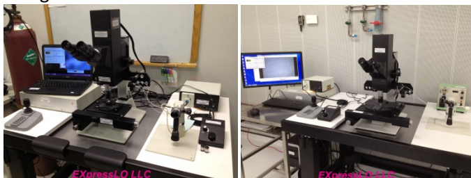
Fully installed 6”x4” motorized stage (left), and 8”x8” motorized stage (right) systems, both configured with 1 manipulator and vibration isolation table.
