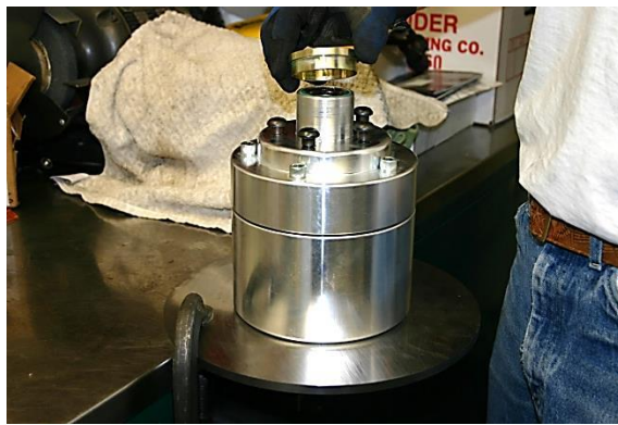
STEP 11: Remove pulley spacer & pulley bolts.
