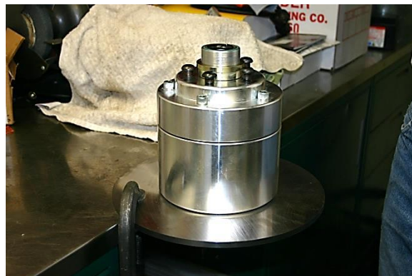
STEP 10: Clamp spool to work bench by rotor.
