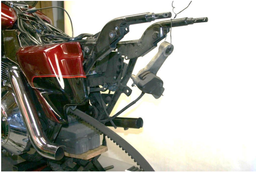
STEP 1: Remove swing arm and fender assemblies.
