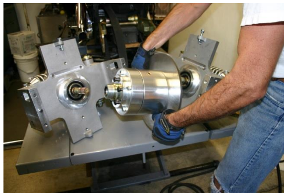
STEP 9: Remove differential spool.
