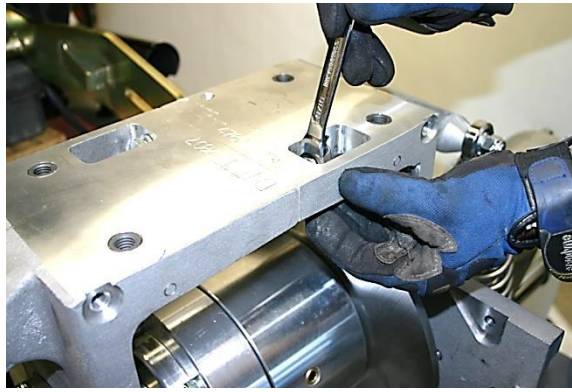
STEP 7: Remove main casting bolts, located 2 top & 2 bottom in milled pockets.
