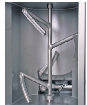
Stainless Steel Feedscrew and Mixing Paddle
