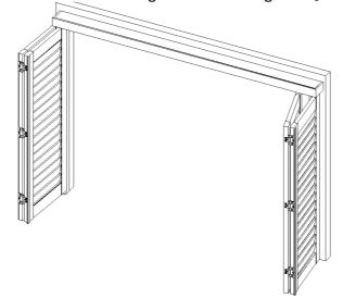
\* Track is pre-installed on the header; standard 1 track only.
