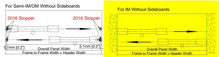
Note: For Semi-Inside/OM bypass without side boards, 2016 Stopper will be supplied.
