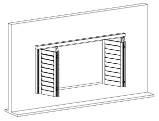
Note: For OM Frame Hinged Bifold shutter not to use as a door, if there is no existing sill at the bottom of the window opening, it is recommended to have the 3" Deco Sill Frame at the bottom.
