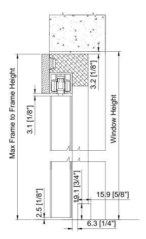
For frame hinged bifold track shutter used as door, the bottom gap will be 3/4" by default. Please specify "Used As Door" on the order form.
