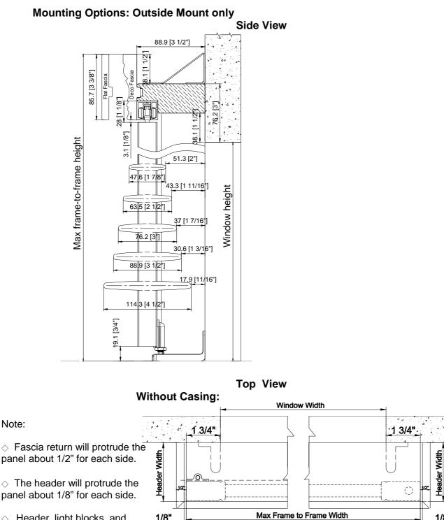
◇ Header, light blocks, and bottom pivot bracket(s) must be installed on a flat surface.
