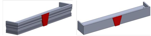
The keystone will be installed by screws. We will pre-drill the screw holes and the screws will be packed in hardware box.
