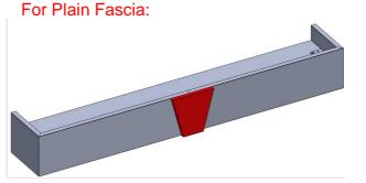
The keystone will be installed by screws. We will pre-drill the screw holes and the screws will be packed in hardware box.
