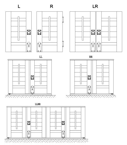
The Panel Lock location for both track system shutters and regular shutters would be the same.
