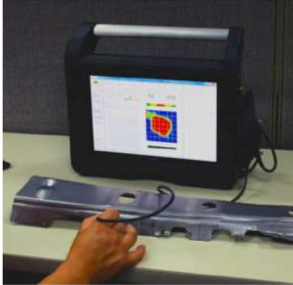
**FIGURE 10.**A portable battery operated MPA ultrasonic inspection unit shown in action.
