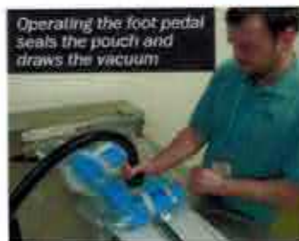
Loading the wrapped tray set into the pouch
