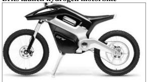
On March 15 the British firm Intelligent Energy introduced its ENV (Emissions Neutral Vehicle) purpose-built, fuel-cell motorbike. At the heart of the machine is Intelligent Energy's 1 kW CORE fuel cell, which can be removed from the bike and used to power other things as needed. A battery pack allows for up to 6 kW peak to the motor
