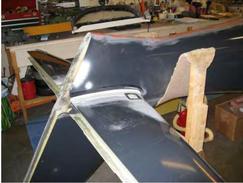
Next is the angle of incidence plates on the wings and another pic of my modified rudder shape, top to bottom.
