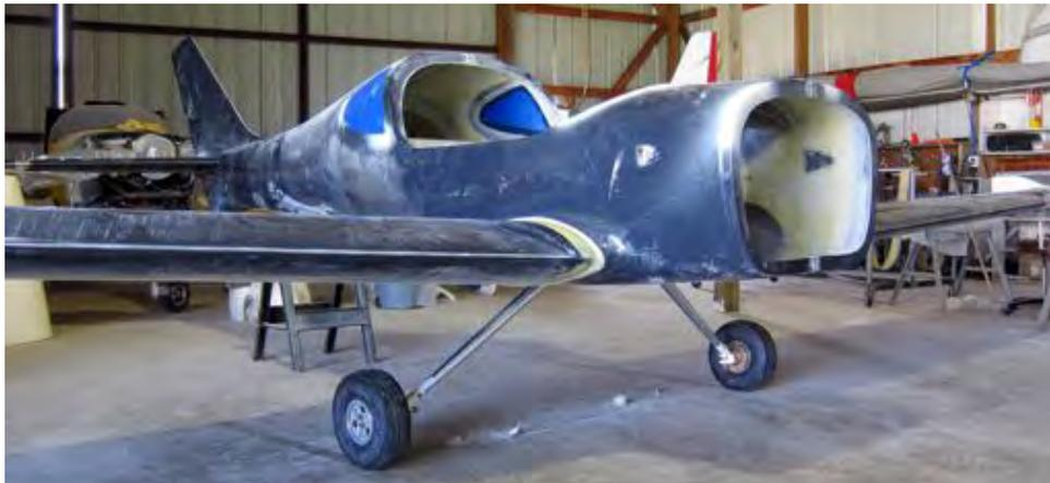
*On the mains after installing and setting toe (week 1)*
