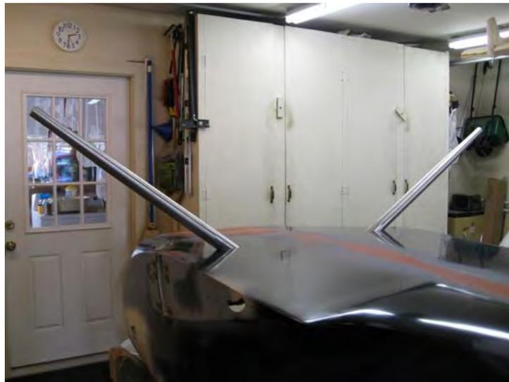
Then another pic of the horizontal tail to fuselage fairings.
