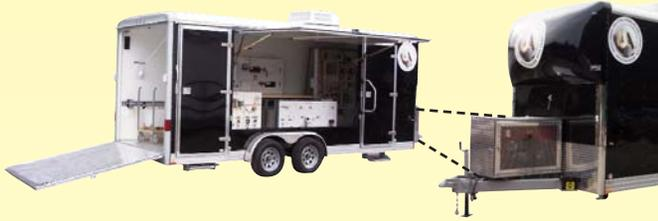
20 ft. With back loading door, open side, two entry doors and generator
