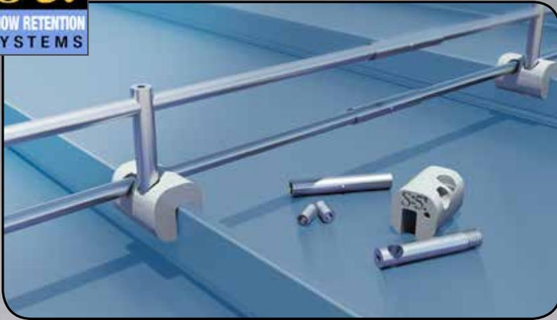
Whether aluminum or brass, our SnoRail™ and SnoFence™ systems offer a sleek, stylish design. Utilizing patented S-5!<sup>®</sup> clamp technology, this snow retention system doesn't pierce the metal roofing, thereby protecting roof coatings and weather-tightness warranties.
