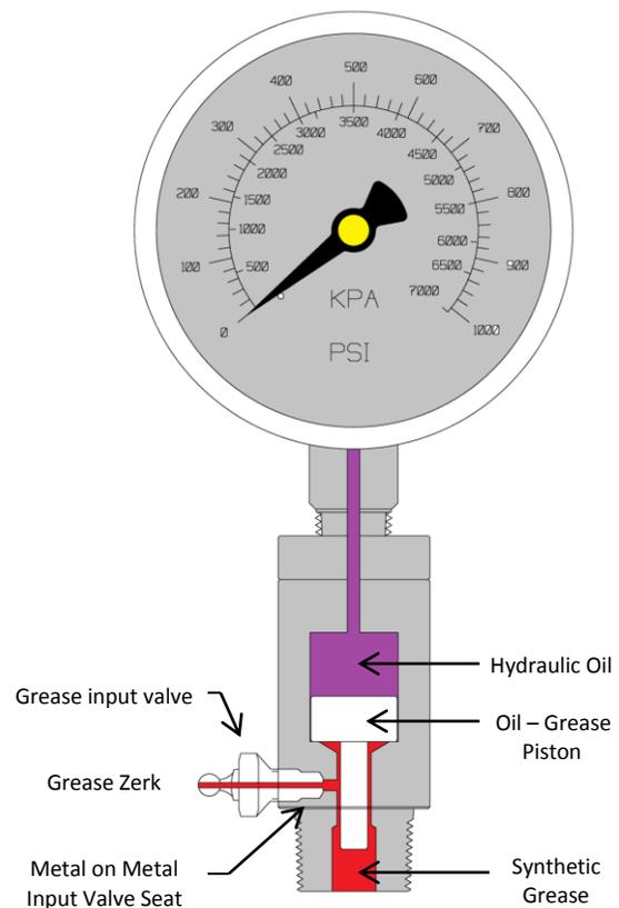
**Gauge Guardian™ is effective in preventing catastrophic process fluid loss under the following conditions:**
