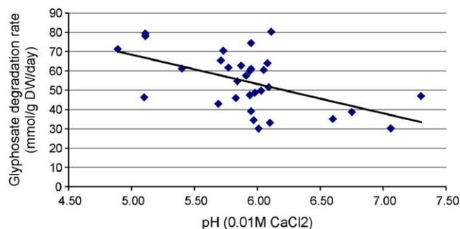
Fig. 4. Glyphosate degradation rates ( $\mu\text{mol/g DW/day}$ ) plotted against soil pH (as measured in 0.01 M  $\text{CaCl}_2$  solution)—significant correlation (Pearson, 0.53,  $P < 0.01$ ), 31 samples.
