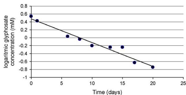
Fig. 1. Representative example of the logarithmic transformed glyphosate concentrations, measured during incubation at 20 °C of a glyphosate–soil suspension, showing the fitted curve.
