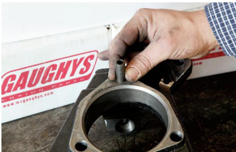
06. Due to the new raised position of the unit bearing to create the 2-inch lowering built into the McGaughys spindle, a stud was used to replace the factory upper retaining bolt. Two of the original three bolts were used to mount the unit bearing and brake dust shield onto the new McGaughys drop spindle. Kelly tightened the included nut onto the stud from the front side with an open-end wrench.
