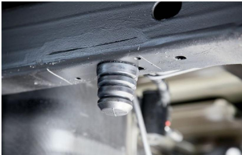
12. McGaughys included multi-stage bumpstops that were bolted onto the frame to provide a measure of safety in case of large suspension impacts while driving.
