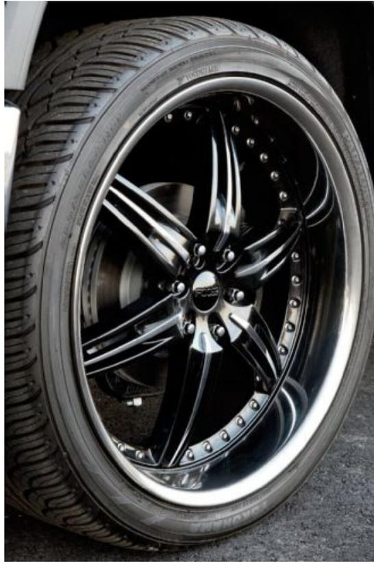
19. Filling the newly lowered wheel openings under the fenders were 24x10 Foose DF-6 wheels finished with black faces and stainless steel lips. Appropriately sized 295/35R24 Yokohama Parada Spec-X tires finished off the look.
