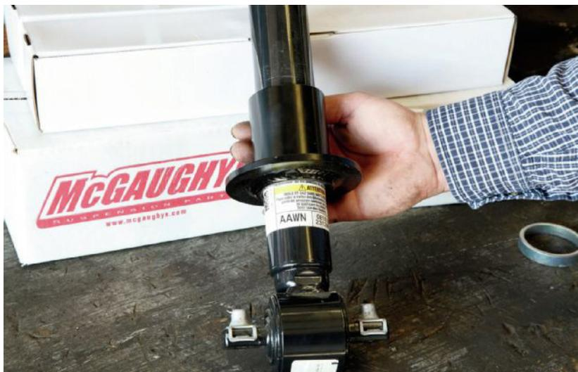
09. It was replaced with the fabricated McGaughys coil cup, which sat lower on the strut body to achieve two inches of drop. Combined with the lowering spindle, the front end was sit a full four inches closer to the ground.
