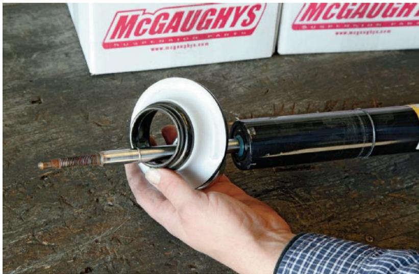
08. Achieving the full four inches of drop required using a spring compressor to disassemble the strut. With the coil spring removed, Kelly knocked the retaining cap off and slid the stock spring cup off the strut.
