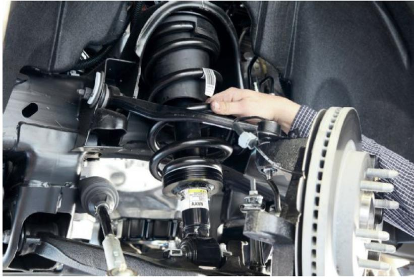
10. Kelly safely reassembled the strut in the spring compressor before placing it back on the '14 Sierra using all of the factory hardware. Since it was now shorter, the strut assembly slid easily into position.
