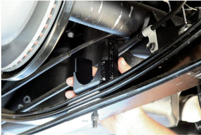
16. Moving the axle on top of the leaf springs created the 7-inch lowering we desired. As part of the suspension kit, these axle saddles located the axle for proper placement.
