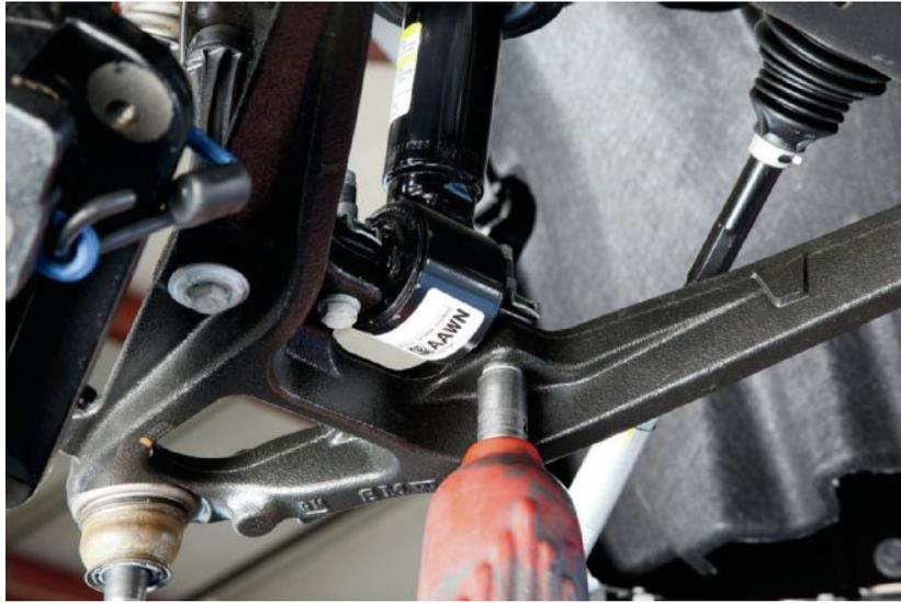
04. Once the three upper retaining bolts were removed with an 18mm wrench (or socket), we moved to the lower strut mounting bolts and zipped them off with a pneumatic gun.
