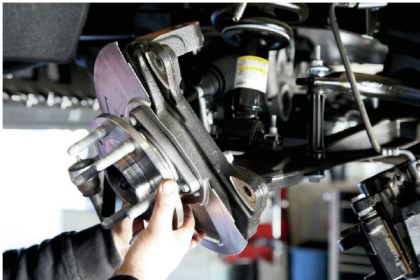
03. Our installer, Kelly, jumped right into the suspension by first pulling the brake caliper and rotor off the factory spindle. Next the balljoints were broken free and the factory spindle was removed from the front suspension.
