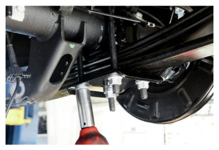
17. Stock U-bolts were torqued in place to keep the GM and McGaughys pieces firmly together for the long haul.
