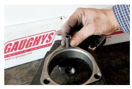
06. Due to the new raised position of the unit bearing to create the 2-inch lowering built into the McGaughys spindle, a stud was used to replace the factory upper retaining bolt.7. Two of the original three bolts were used to mount the unit bearing and brake dust shield onto the new McGaughys drop spindle. Kelly tightened the included nut onto the stud from the front side with an open-end wrench.
