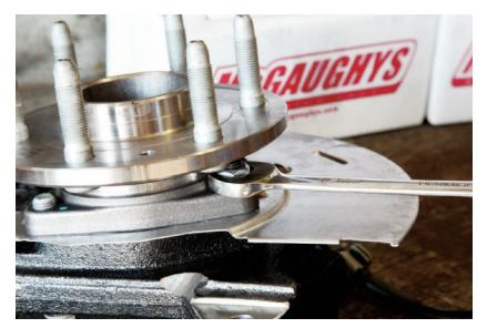
07. Two of the original three bolts were used to mount the unit bearing and brake dust shield onto the new McGaughys drop spindle. Kelly tightened the included nut onto the stud from the front side with an open-end wrench.
