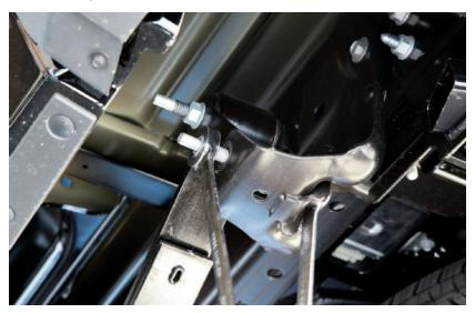
15. Using a couple of 21mm wrenches, Kelly removed the lower shackle bolts all together and only loosened the upper shackle bolts for freedom of movement.
