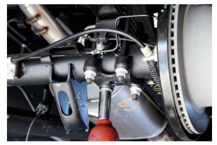
13. Both rear shocks were removed and discarded, as they'll be upgraded with improved units from McGaughys. Safety stands were used to support the axle while Kelly zipped off the U-bolts.
