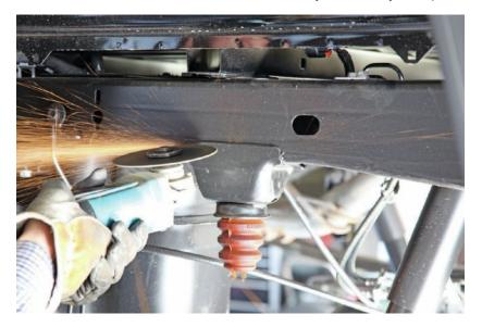
11. For the rear suspension, an axle flip was performed to achieve the desired seven inches of lowering. Kelly attacked the bumpstop mounts with an electric cut-off wheel to remove them for axle travel clearance.
