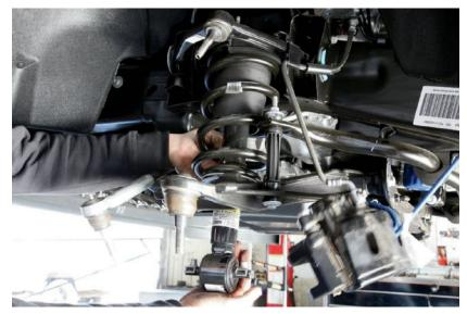
05. Kelly lowered the complete stock strut assembly from the Sierra without much fanfare or unnecessary labor.
