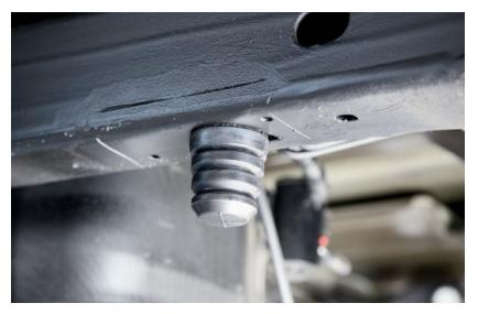
12. McGaughys included multi-stage bumpstops that were bolted onto the frame to provide a measure of safety in case of large suspension impacts while driving.
