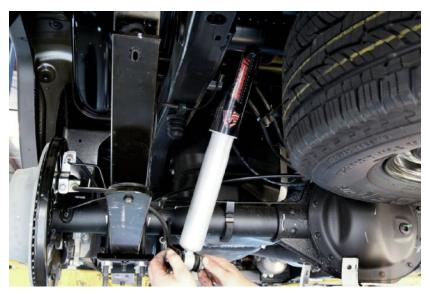
18. Instead of adding shock extenders, McGaughys supplied us with a pair of its gas-charged performance shocks designed especially for this application.
