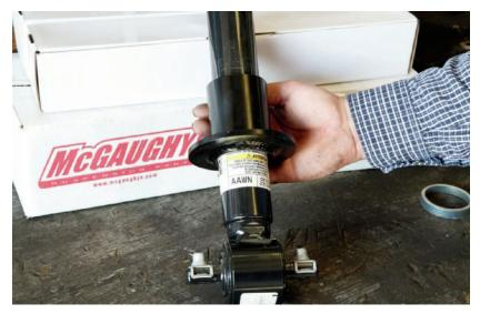
09. It was replaced with the fabricated McGaughys coil cup, which sat lower on the strut body to achieve two inches of drop. Combined with the lowering spindle, the front end was sit a full four inches closer to the ground.
