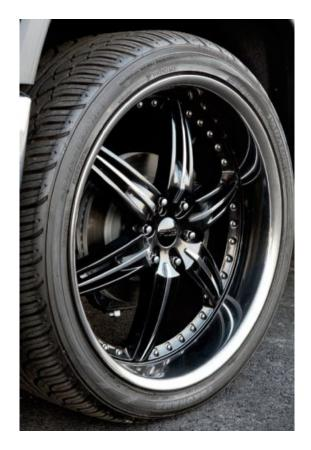
19. Filling the newly lowered wheel openings under the fenders were 24x10 Foose DF-6 wheels finished with black faces and stainless steel lips. Appropriately sized 295/35R24 Yokohama Parada Spec-X tires finished off the look.
