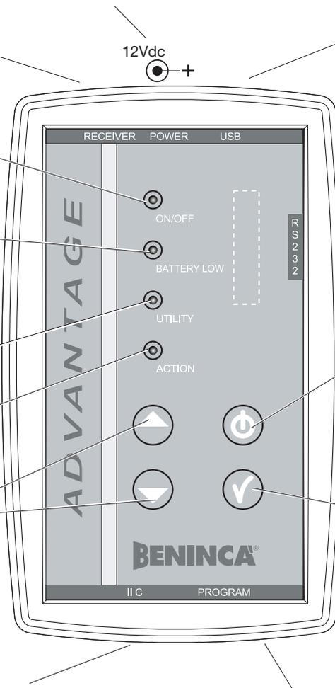
The ADVANTAGE palm programmer is central core of the system, since it acts as a communication interface between the "Advantage" software installed on the computer and the radio components (i.e. receivers and transmitters). It has a built-in receiver for 433.92MHz rolling code transmitters, which can store up to 2048 transmitters. This receiver acts as buffer memory to contain the data read by another receiver or by an Advantage file resident on PC.
