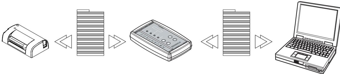
So the internal memory of the programmer acts as interface between receiver and software allowing files to be transferred from receiver to PC and vice-versa.
