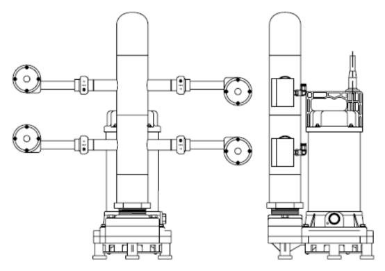
Units are connected in parallel to main outlet pipe which has larger diameter pipe than the pipe to TR6242 to maintain even pressure to each unit.
