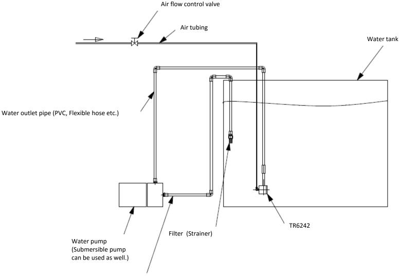
Water inlet pipe (PVC, Flexible hose etc.)
