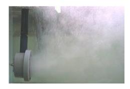
Pump requirement: Minimum pressure of 0.1Mpa at 30 l/m water flow rate The air volume is up to 15% of water volume.
