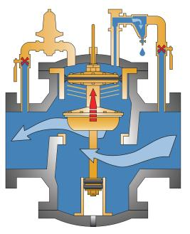
If the main valve <u>does not respond</u> to manual operating, it usually indicated that the packings need to be replaced. Typically, the condition of the packings can be accurately gauged by observing the leakage through the vent hole in the bottom cap of the main valve. Negligible leakage usually indicated that the packings are serviceable.
