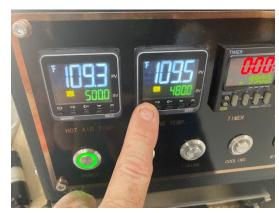
PRESS THE CIRCLE KEY (LEVEL KEY) ON FAR LEFT SIDE OF OMRON AND HOLD IT UNTIL MENUS SETTINGS APPEAR (3 SECONDS)
