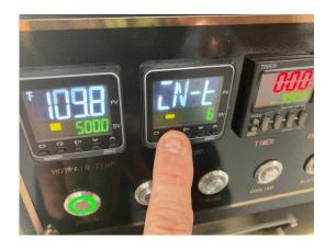
2. THE FIRST MENU SETTING WILL APPEAR. NEXT PRESS THE 2ND KEY FROM LEFT ONCE WHICH IS THE MODE KEY. (FIRST PARAMETER SETTING IS:IN-T SETTING= IMPORT TYPE)
