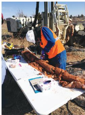
Sonic soil cores are examined in the field by an onsite geologist. The cores were retrieved by running SDT60 and an 8150LS.
