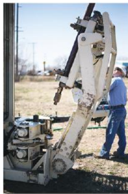
Running sonic weighted wireline with SDT45 tooling. (above) Modular weight assembly, with the overshot 'spear' visible inside the weight head prior to being lowered downhole. The modular weight assembly consists of two, 150-lb. weight segments coupled together and a threaded head and overshot spear.
