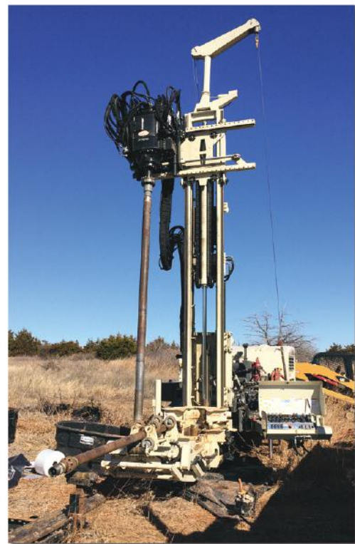
An 8150LS Rotary Sonic, owned by Associated Environmental Industries in Norman, OK, is running SDT60 and a 6.0-in. Weighted Wireline system.
