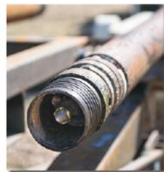
Running sonic weighted wireline with SDT45 tooling. (above) Modular weight assembly, with the overshot 'spear' visible inside the weight head prior to being lowered downhole. The modular weight assembly consists of two, 150-lb. weight segments coupled together and a threaded head and overshot spear.
