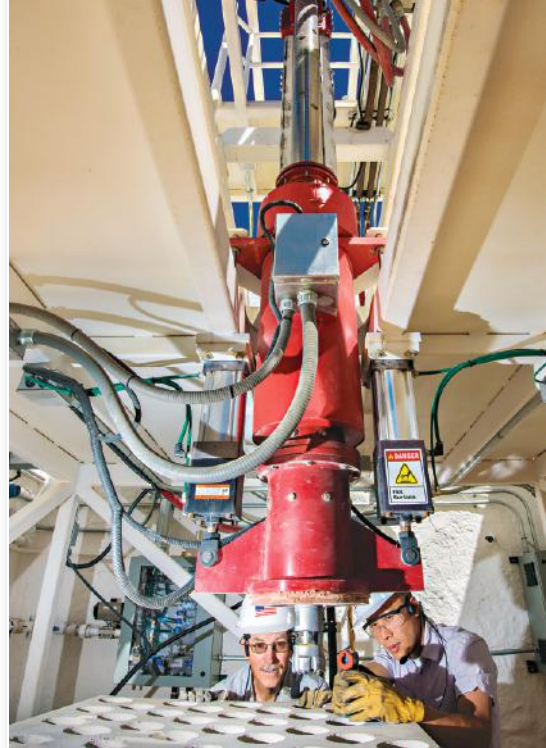
Technologist Elton Wright assists as Jiann Su inspects a down hole hammer used at the HOT test facility. Photo by Randy Montoya.
