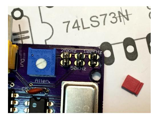
Also seen in this photo is a preset potentiometer, this is designed to vary the output level and if required to trim the square wave as needed, when the calibrator is connected to a scope. This is factory preset, so should not require any user adjustment.
