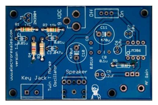
Stage 1 – Insert all resistors (R1,R2,R3,R4 & R5) - compare to this picture
