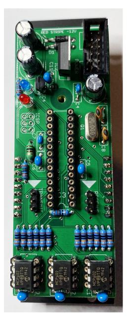
Install the ATMEGA328P CPU into IC3 socket. After a final check of all work for shorts, missing or poor solder joints etc, next join the boards together and secure with the 6mm M3 screw. Please refer to the user guide for instructions on connecting your Parasite to its Amoeba host.
