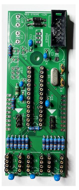
Install and solder the two LEDs, RX and TX. The picture below shows the orientation: the anode (+) is the longer pin and the cathode (-) is the shorter pin.
