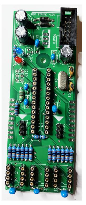
Install and solder the 7805 voltage regulator IC2 and the 7905 voltage regulator IC4. Pay close attention to the orientation on the silkscreen and the picture below.
