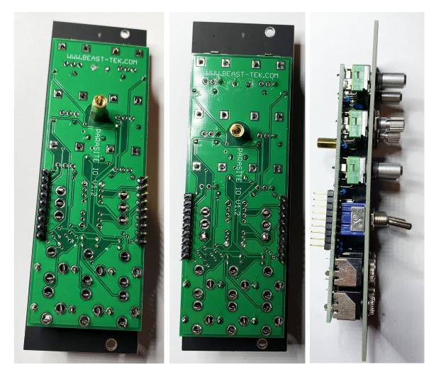
Now that everything is seated nicely, solder the rest of the pins. Pay close attention to the 1P4T switches – you don't want to solder the single pin holding it in until last – heating that pin will make the switch fall out and you will need to go back to step 1. Slowly and carefully solder the pins of the 1P4T switches – they are sitting flush with the bottom of the PCB so make sure you get a good solid solder joint.
