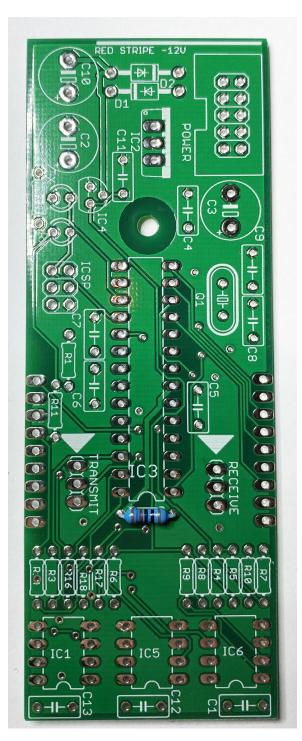
Install and solder the two 220R resistors R11 and R12.
