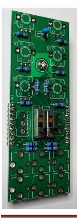
Seat the potentiometers, SPDT switches and jacks carefully on the PCB. Do NOT solder yet.
