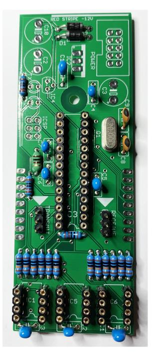
Install and solder the power header.
