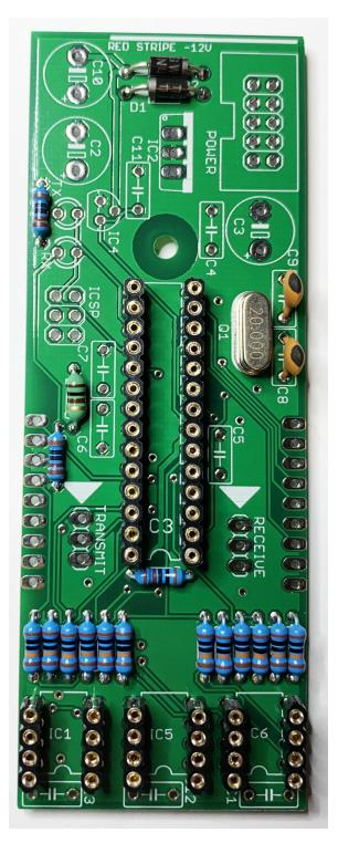
Install and solder the eight 100nf capacitors C1, C4, C5, C6, C7, C11, C12 and C13.
