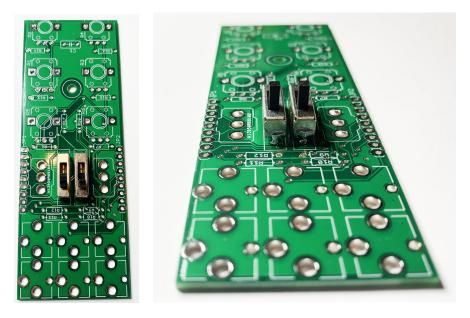
Once the soldered, reheat and adjust the switches so that they are at right angles and will align with panel. DO NOT solder any more pins until right at the end – **just in case you need to adjust them.**
