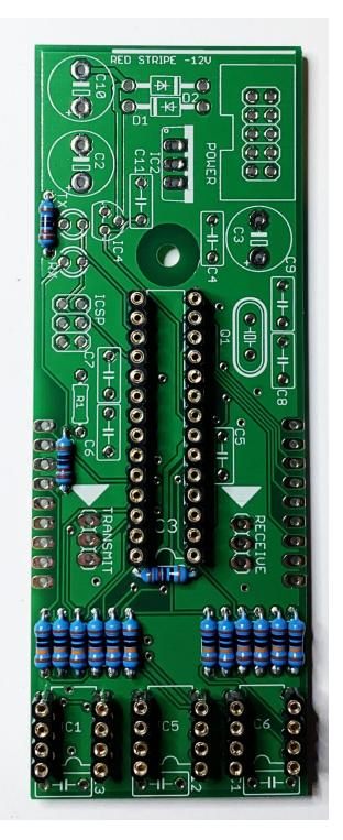
Install and solder the 20mhz crystal Q1.
