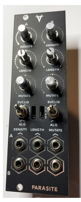
Place four jack nuts on to the outer jacks finger tighten only. Place washers and nuts onto the two T18 potentiometers and again finger tighten only. This should create enough tension so that you can flip the board over without everything falling apart. You may have to add additional nuts on to the pots if this is not the case.
