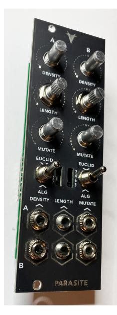
Flip the module over (gently!) and solder one pin of each jack, pot and switch. Flip the module on its side and make sure everything is sitting flush and neatly. If something is misaligned, you can reheat the single pin and make adjustments as necessary.
