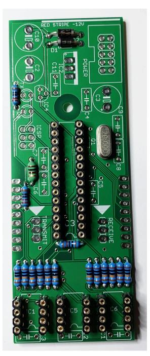
Install and solder the two 22pf capacitors C8 and C9.
