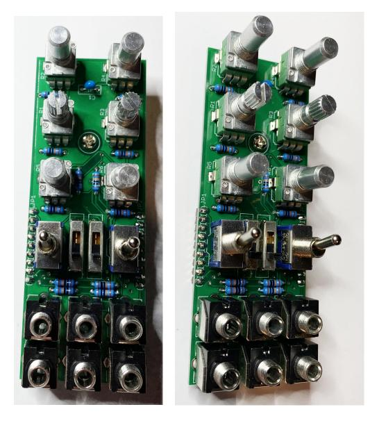
Carefully slide the panel over the components. Place the nuts onto the SPDT switches and **finger** tighten.
