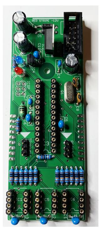
Cut two nine pin pieces of female header socket from the female header strip. Install and solder into place.
