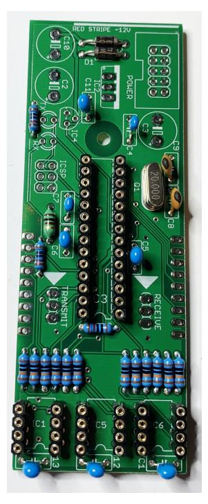
Cut two three pin pieces from the male header strip. Install and solder into "TRANSMIT" and "RECEIVE".
