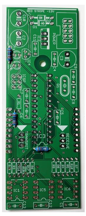
Install and solder the twelve 100K resistors R3, R4, R5, R6, R7, R8, R9, R10, R14, R16, R17 and R18.
