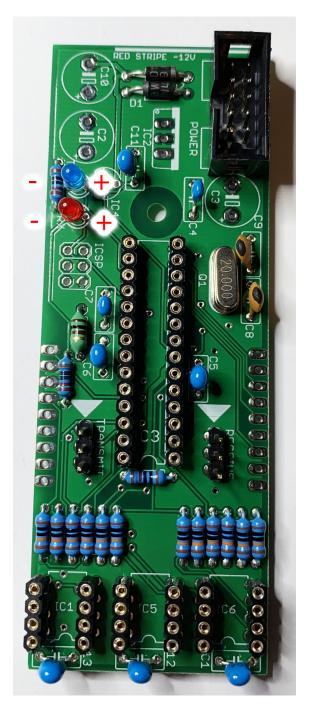
Install and solder the two 100uf capacitors C2 and C10 along with the 10uf capacitor C3.
