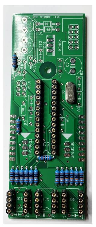
Install and solder the two 1N4004 power diodes D1 and D2 along with the 100uh inductor R1.
