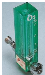
Low-pressure flowmeters: (Left) A pressure-compensated flowmeter; (Right) a constant flow selector valve.
