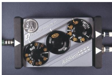
An automatic transport ventilator. The coin is shown for scale. © Edward T. Dickinson, MD
