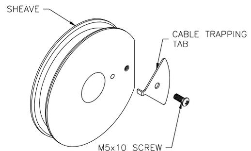
**Fig 11b-Cable Trapping**
