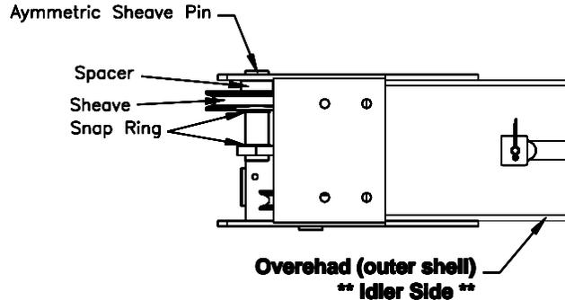
Fig 7 – Asymmetric Sheave Assembly
