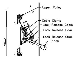
Fig 13 - Power Side Lock Release Assembly
