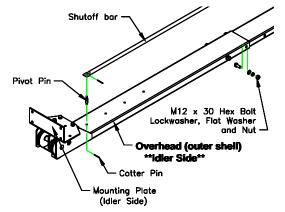
Fig 5 – Symmetric Overhead Assembly
