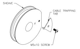
Fig 11b-Cable Trapping
