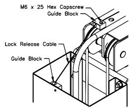
Fig 12 - Idler Side Lock Release Assembly
