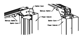
Fig 9 –Limit Switch Cord Routing
