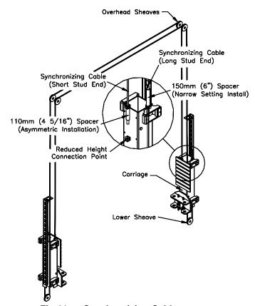
Fig 11a - Synchronizing Cables
