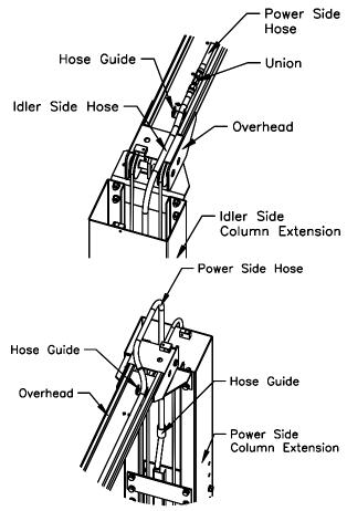
Fig 10 - Hydraulic Hose Routing
