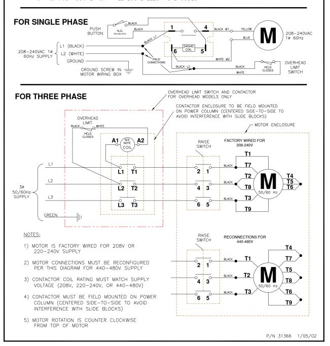
Fig 15 - Electrical Wiring Diagram
