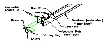
Fig 6 – Asymmetric Overhead Assembly
