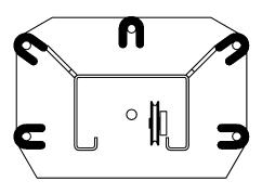
Fig 4 - Column Shimming
