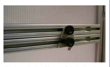
Our camlocks consist of an aluminum body with at radial slot that is not concentric to its pivot point. The farther you push, the tighter it squeezes the panels together. We implement thumb screws and t-nuts to make the **installation very simple without the use of tools**. The picture above shows how we machine slots into the extruded panel frames to allow for a quick installation of the camlock assembly.
