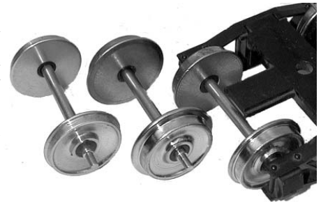
NWSL #1 gauge wheelsets—1 to r: /172, /270, /236 treads on standard shouldered axle
