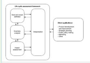
Stages of an LCA as per ISO 14044:2006. Click here to see larger version of the diagram.
