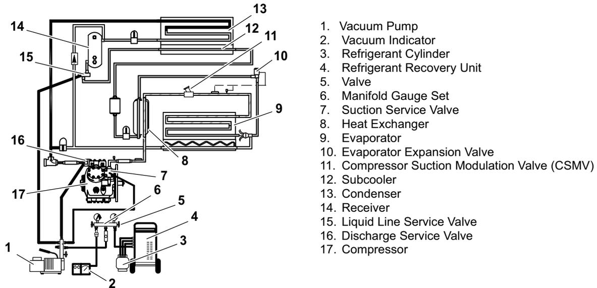
**Figure 8.23 Four Port Manifold Gauge Option**
