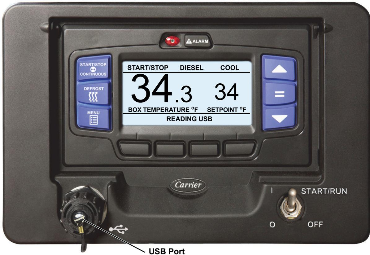
1. Data may be downloaded with the system powered up or turned off. Remove protective cover from the USB interface port and insert the Carrier Transicold APX USB Flash Drive, CTD P/N 12-00814-00. The MessageCenter will display READING USB.
