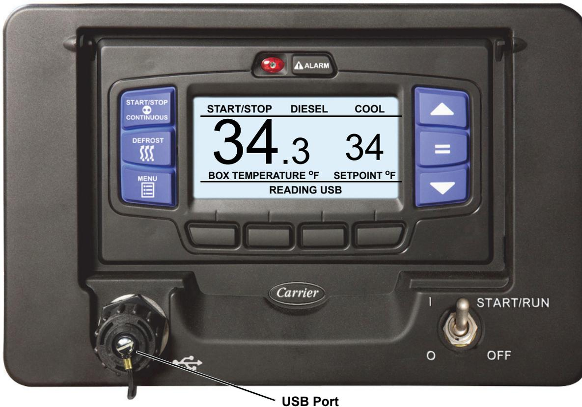
1. Ensure the desired software version folder is the only folder loaded in the “PROGRAM” folder on a data transfer USB memory device.
