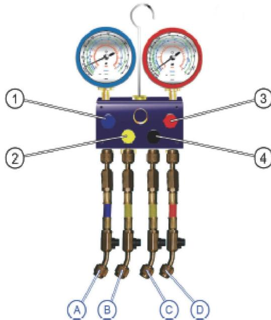
1. Connect the manifold gauge set to the unit (refer to [Figure 8.25](#))
