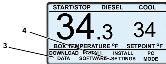
5. If one or more configuration file(s) are loaded on the data transfer USB memory device a listing of available files will be displayed. To scroll through the files press the ▲ or ▼ key. The files will highlight as the list is scrolled.
