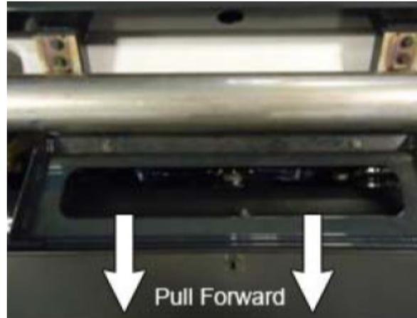
7. Remove the upper fan shroud bolts, and remove the shroud.
