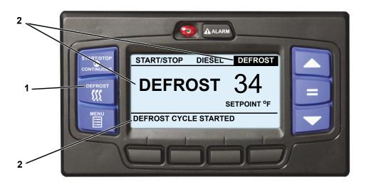
1. With the system powered up (START/RUN-OFF switch in the START/RUN position) press the MANUAL DEFROST key.
