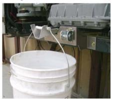
Figure 8.12 Oil Drain Tool
