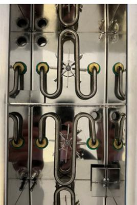
Advanced stirring by a propeller in each section ensures homogenous dye mixture and temperature.
