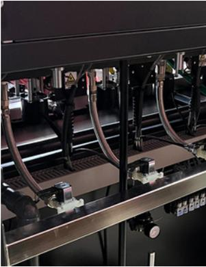
Integrated automatic fill\* and drain system with a 3-way valve ensures economy and a fast process.
