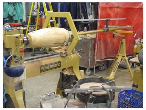
First, this article covers hollowing to depths that commercial boring bars will not go, in excess of thirty inches (76.2 CM) deep. The deeper/bigger you go, the difficulty/danger expands exponentially. <u>Also, DO NOT forget how dangerous it is to have several hundred pounds of</u> rotating mass in your lathe, which can turn lethal in a heartbeat!)
