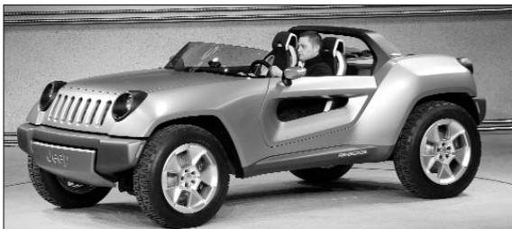
The Jeep Renegade Concept (above) has one 200 kW (268 hp) motor per axle, with low range and locking differentials, a 16 kWh li-ion battery pack, and a 1.5 liter 3-cylinder BLUETEC diesel as a range extender, supplied by a 10-gallon fuel tank. With this much power it has a bit more perfor-
